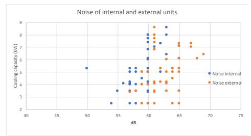
**Figure 1.** Topten: Distribution of noise value for indoor and outdoor units according to their cooling capacity
